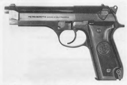
Original Beretta entry as U.S. service sidearm, M92S had rotating firing-pin safety but Army barred butt mag-release button. Photo: Beretta
